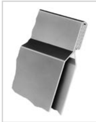
Fig. 3-2: Folded connections give the exchanger package severalfold material thickness for the leading and trailing edges (design N shown here).
