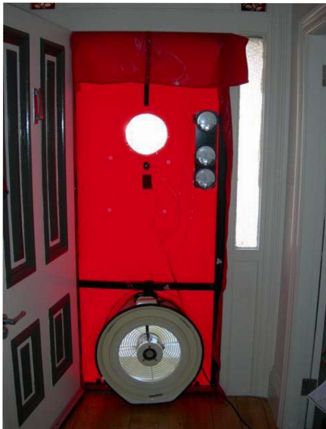
Blower door in test environment.
