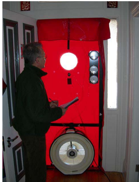
Blower door measurements being taken.
